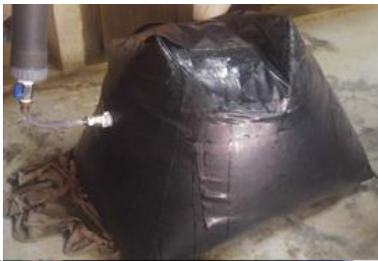
Fig 12: (Left) Water Tight test on Gas Storage. (Right): Mounted system after various test.
