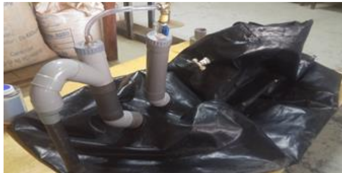
Fig 12: (Left) Water Tight test on Gas Storage. (Right): Mounted system after various test.
