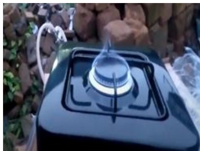
Fig23: Burning test of biogas from prototype digester.
