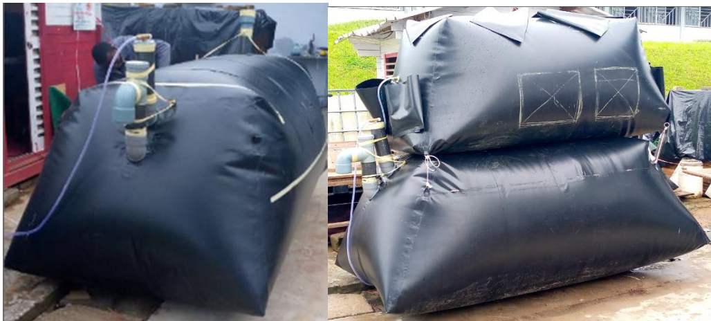
Fig 25: Successful HDPE geomembrane bio-digester ready for installation
