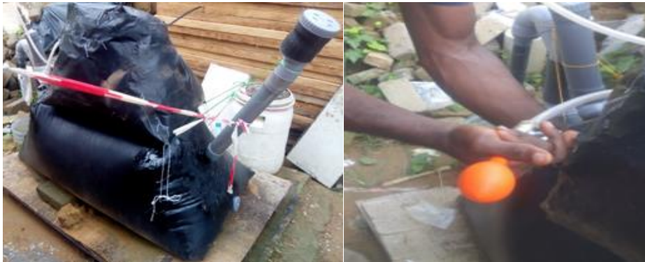
Fig 15: (Left): Prototype bio-digester after HRT; (Right): Gas sample collection.
