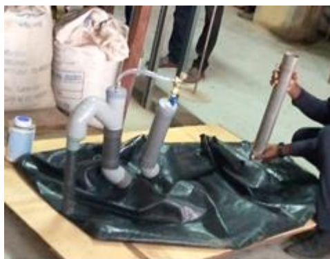
Fig 10: Complete 300L prototype bio-digester ready for feeding
